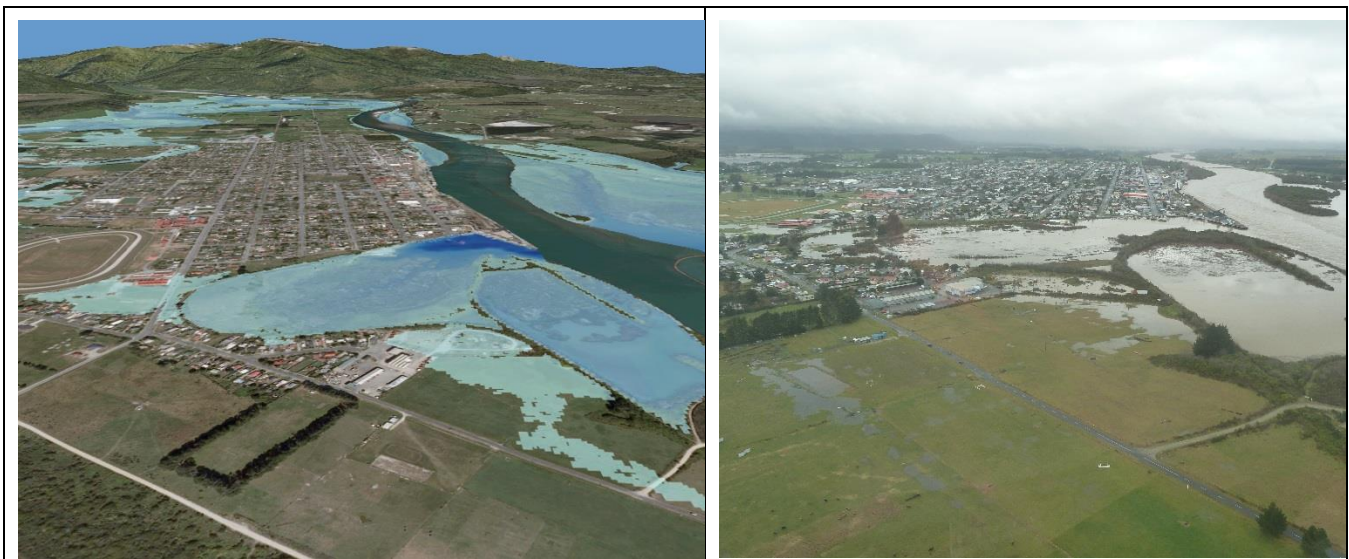
Figure 3-21 - Comparison of calibration results with aerial photography upstream of the Buller River mouth
